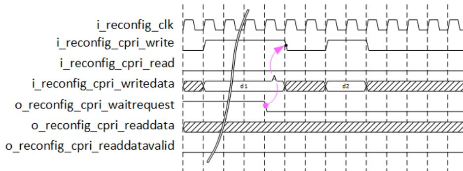
Figure 15. Reading from CPRI PHY Reconfiguration
